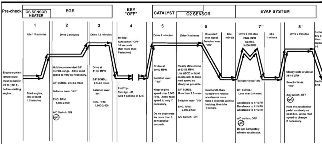
**NOTE:** It is better to perform this driving test when fuel level is less than 1/2. If fuel level is greater than 1/2 more time may be required to complete EVAP sections of the drive pattern. Also you may be unable to add fuel as required.
