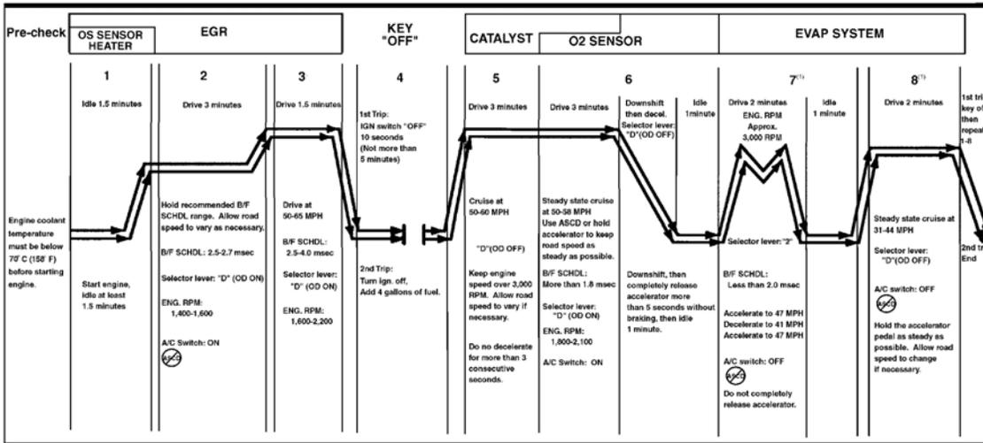
**NOTE:** It is better to perform this driving test when fuel level is less than 1/2.
